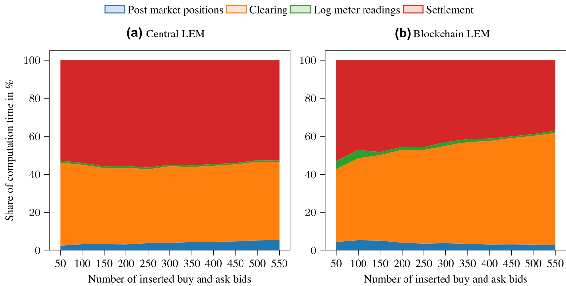
FIGURE 3 Share of computation time used for the main Local Energy Market (LEM) functions: posting bids, market clearing, meter reading logging, and market settlement in the blockchain-based and central LEM
