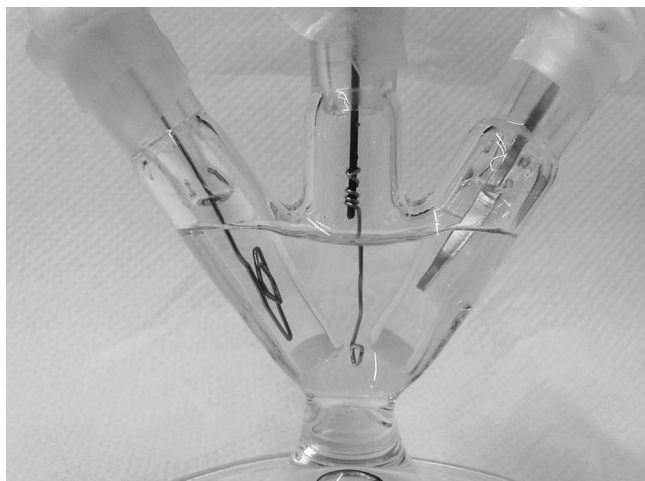
Figure 1. Three-electrode glass setup with a Pt CE (left) and a Au WE (center) in EC:DEC (1:1 w:w) electrolyte containing \text{LiClO}_4 concentrations from 0.1 \times 10^{-3} to 2 M and 50 \mu\text{M} Fc (ferrocene) as well as a metallic Li RE (right) in the same electrolyte without Fc.
