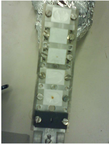
Figure 2. Photographed image of the ^{64}\text{Zn} target on the MLL target ladder shortly after the experimental run.
