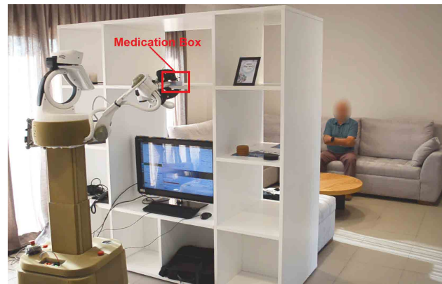
Figure 1. The RAMCIP robot engaged in a real medication adherence assistive task with a user in an actual home environment.
