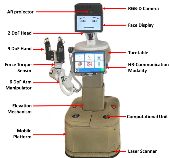
Figure 2. The basic architectural elements of the RAMCIP robot. The robotic platform with the elevation mechanism, the turntable, the arm manipulator and the head have been developed by ACCREA Engineering ® . The utilized hand is the smart grasping system of SHADOW Robot Company, Ltd. ® .
