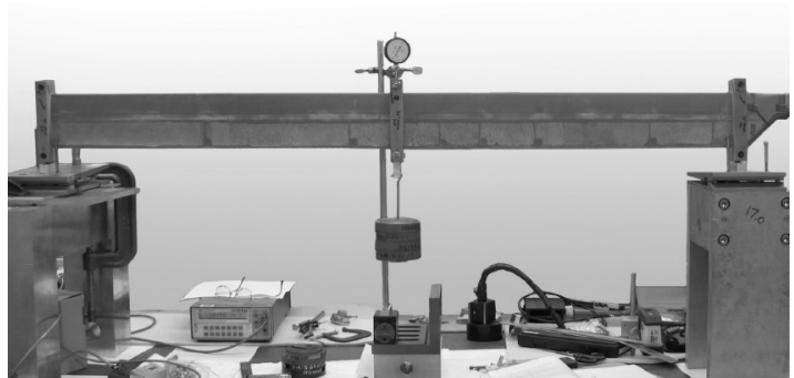
(a) Cantilevered bending test of the IRI T22/T23 rotor blade with photogrammetry. Adapted from [19]. (b) 3-point bending test of the HART-1 rotor blade. Adapted from [78].
