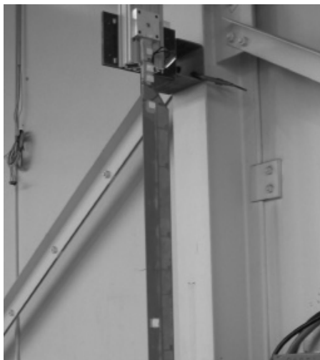
(a) HART I flap bending experiment using the mirror method. Adapted from Jung et. al. [78] (b) Digital inclinometer measurements to determine the torsional twist angle. Adapted from Jaksch [75].
