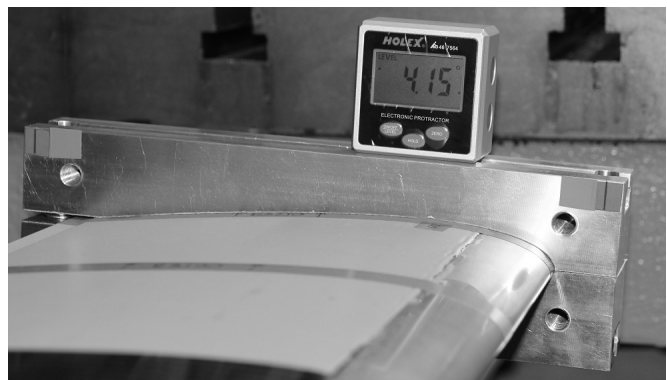
(a) HART I flap bending experiment using the mirror method. Adapted from Jung et. al. [78] (b) Digital inclinometer measurements to determine the torsional twist angle. Adapted from Jaksch [75].
