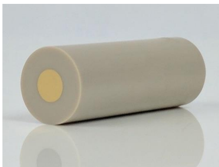
Figure 3.5. Photograph of a gold rotating disk electrode (5 mm diameter). Adapted with permission from ref. [169].
