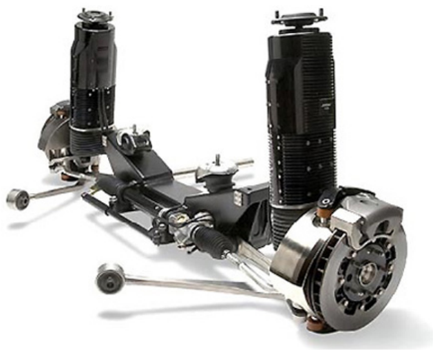
Figure 2.8: Bose active suspension [97]
