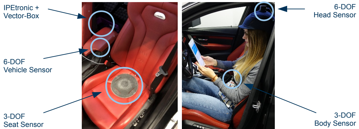
Figure 5.2: Measurement system installed in the simulator mock-up, with and without a seated test person
