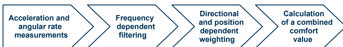
Figure 2.4: Basic principle of standardized vibration assessment methods according to ISO 2631 [29], BS 6841 [30] and VDI 2057 [31]
