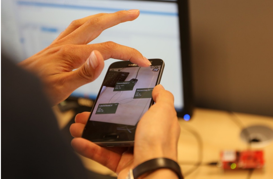
Figure 5.1: Hand-held AR device superimposes the camera image of the physical IES with device information and network traffic flows represented as arrows between devices
