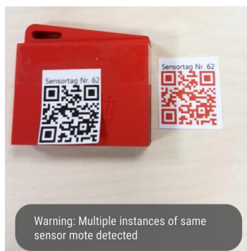
Figure 5.6: Duplicate QR codes in the camera field of view (FOV) raise a warning.
