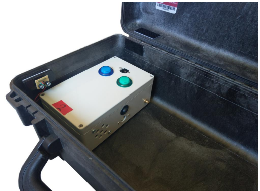
Figure 4.9: Box prototype v3 with miniaturized electronics.
