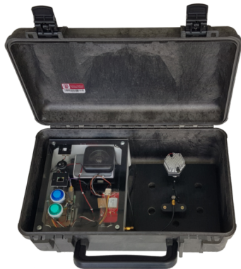
Figure 4.8: Box prototype v2 utilizing a COTS Faraday Cage.
