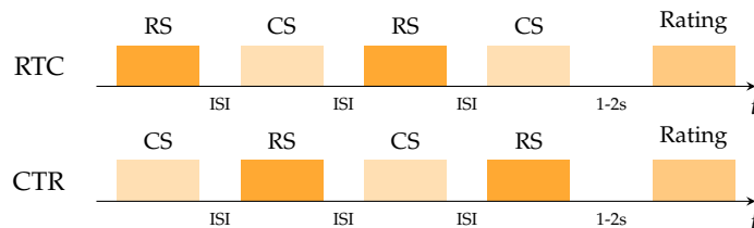
Figure 4.7 Trial for evaluating the quality of one compressed signal (CS) compared to the reference signal (RS) for the two different run types reference-then-compressed (RTC) and compressed-then-reference (CTR). Adapted from [4] © IEEE 2021.
