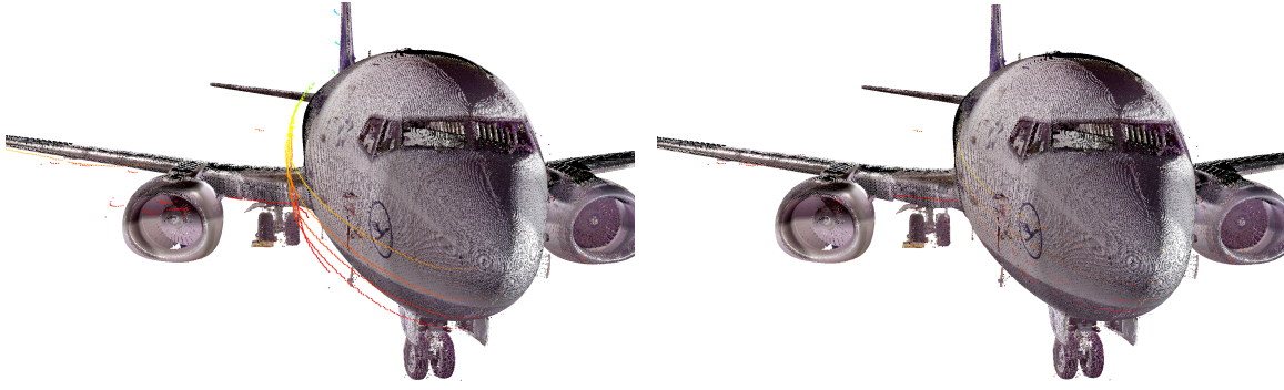
(a) Isolated LiDAR scan before the scan-to-model alignment. The offset is due to the error in the map-optimized pose. (b) Isolated LiDAR scan after 100 iterations of scan-to-model alignment. The scan is fully aligned to the model surface.
