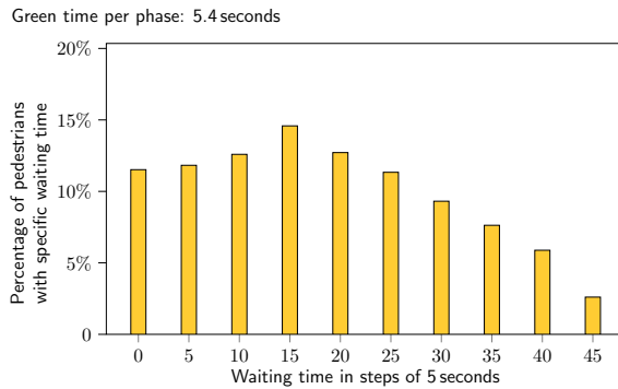
(a) Histogram of ped. waiting times in steps of 5 seconds for t_{sig}^{green}=5.4 seconds and symmetric vehicle demand x=2,000 .
