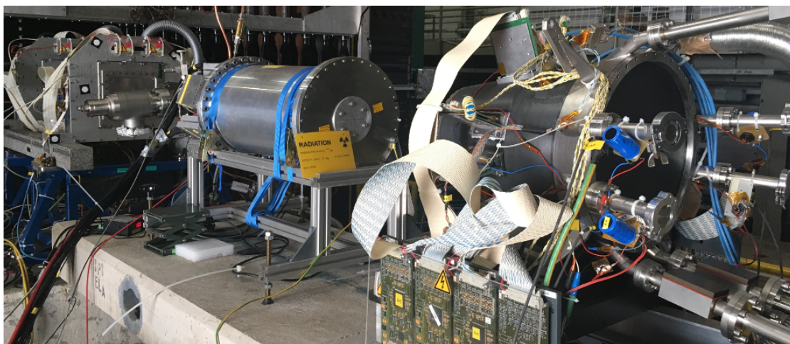
Figure 2.1: Setup of the feasibility test at COMPASS. The TPC is visible in the center surrounded by silicon-microstrip tracking detector up- and downstream.
