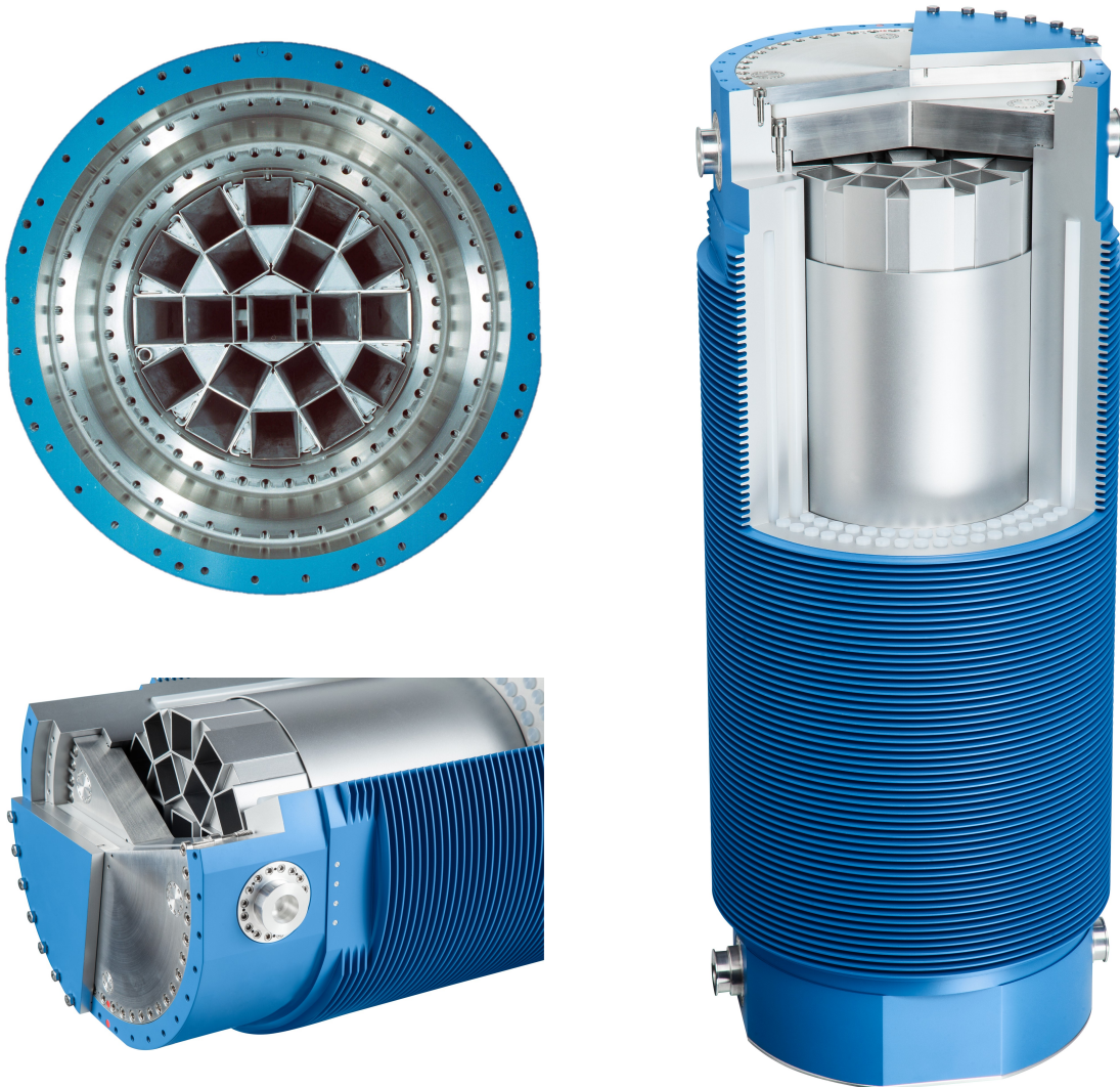
Figure 2.10: CASTOR ® V/19 cask from GNS. On the upper left picture, we can see the configuration of the basket and 19 fuel assemblies in the cask cavity. On the lower left picture, we can observe the closing system including a primary lid and a secondary lid. A protection plate (blue painted) comes on top of the double-lid system. The two rows of polyethylene moderator rods (white rods and round spots in the cask body) can be seen on the vertical cask. On the external surface of the cask, cooling fins are used to enhance the heat removal. Taken from [28].
