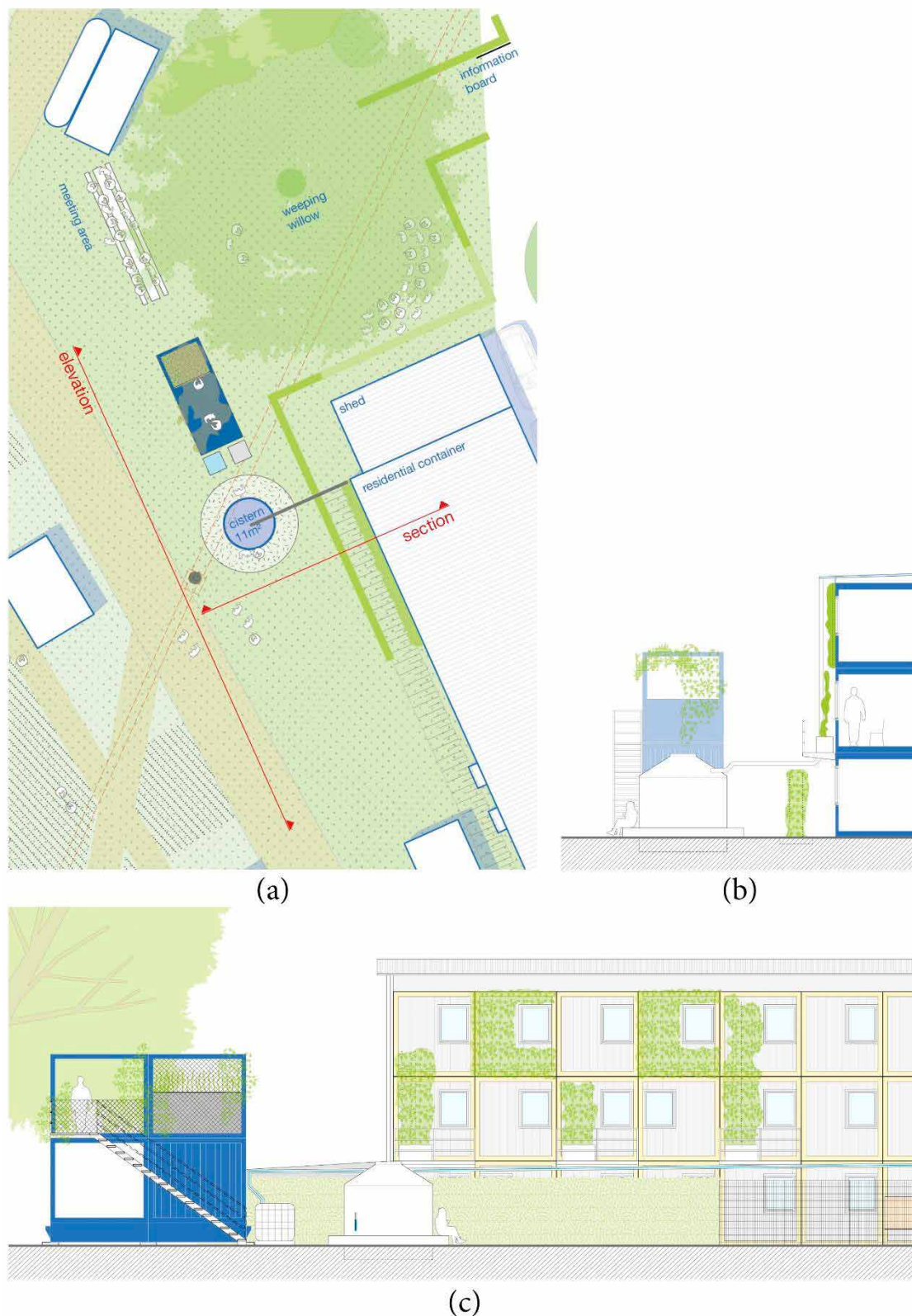
Figure 8. Design Variant V 13 (no scale) as a basis for discussion and elaboration with the specialist planners: (a) site plan; (b) section through residential container and façade greening; (c) elevation of two-storey container module, cistern and façade greening.
