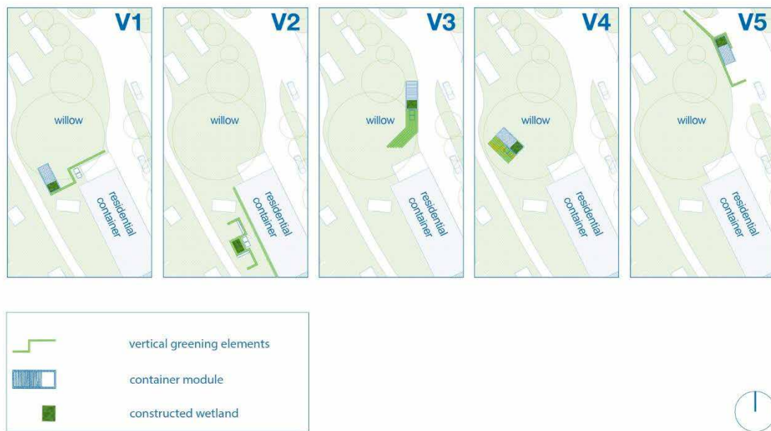
Figure 5. Design variants V 1–5 (no scale), all consisting of one or two container modules, a constructed wetland and various options for vertical green elements. The architect’s initial conceptual considerations show a range of options for the planned location and design of the Impulse Project.
