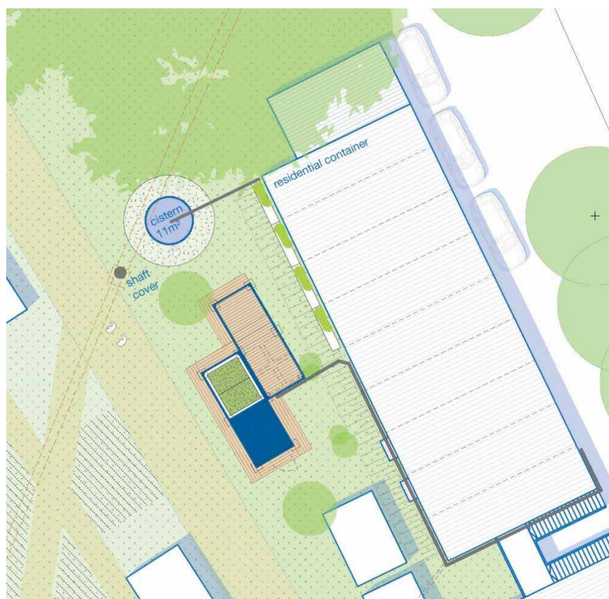
Figure 9. Final design variant V 16 (no scale). The single-storey solution consists of two container frames housing the technical room, the constructed wetland and two terraces, of which one is on top of the grey water storage tanks.
