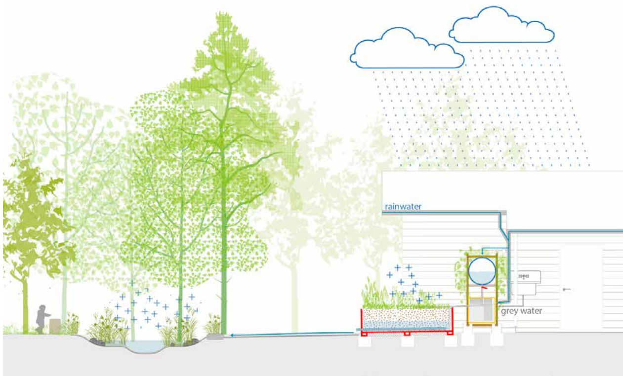
Figure 11. Final design of the blue-green greywater treatment system. The greywater from the kitchen sink (not shown in the picture) and the outdoor sink (on the right) is pre-cleaned in the septic tank (yellow). The roof runoff flows via the rainwater storage tank (blue) to the filtration bed and is fed directly in case of heavy rainfall. The timber frame that supports the septic tank and the rainwater storage tank is overgrown with climbers. The insulated filtration bed is filled with lava sand and grown with flowering marsh plants. The treated water is directed to the frog pond via an open gutter. The pond is planted in the shore area and has a nature observation place for the pupils.
