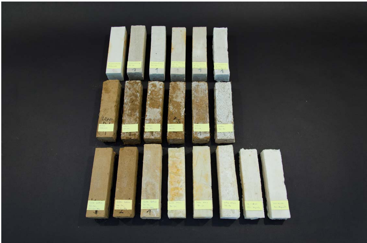
Figure 18. The first test specimens of salt and the different binders (source: Vesna Pungercar).
