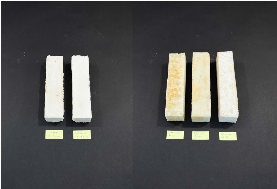
Figure 21. The salt + corn starch test specimens with different mixing ratios (from left to right): 86.0% salt + 13.0% Ca-Alginate, 90.0% salt + 5.0% Ca-alginate, 70% salt + 30% corn starch, 80% salt + 20% gypsum, 90% salt + 10% corn starch.
