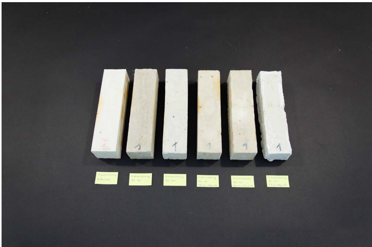
Figure 19. The test specimens of salt, gypsum and Ca-alginates with the different mixing ratio (from left to right): 0.0% salt + 100.0% gypsum, 30.0% salt+70.0% gypsum, 20.0% salt + 80.0% gypsum, 30.0% salt + 70.0% gypsum + 5.0% Ca-Alginate, 30.0% salt + 70.0% gypsum + 10.0% Ca-alginate, 30.0% salt + 70.0% gypsum + 15.0% Ca-Alginate.
