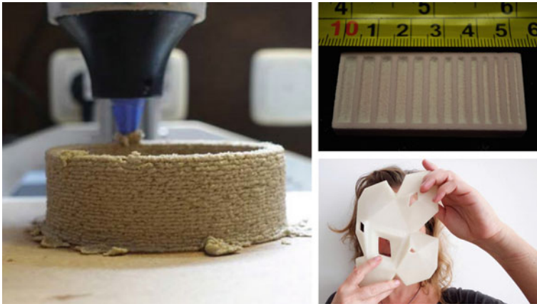
Fig. 3 Left—additive manufacturing. Right above—the first 3D printing salt prototypes. Right below—the 3D-printed salt part for a 3D-printed salt pavilion. Source Left—TUM EBB. Right above—The Solheim Additive Manufacturing Laboratory of the Mechanical Engineering Department of the University of Washington [68, 69]. Right below—Emerging Objects/Ronald Rael and Virginia San Fratello [71]
