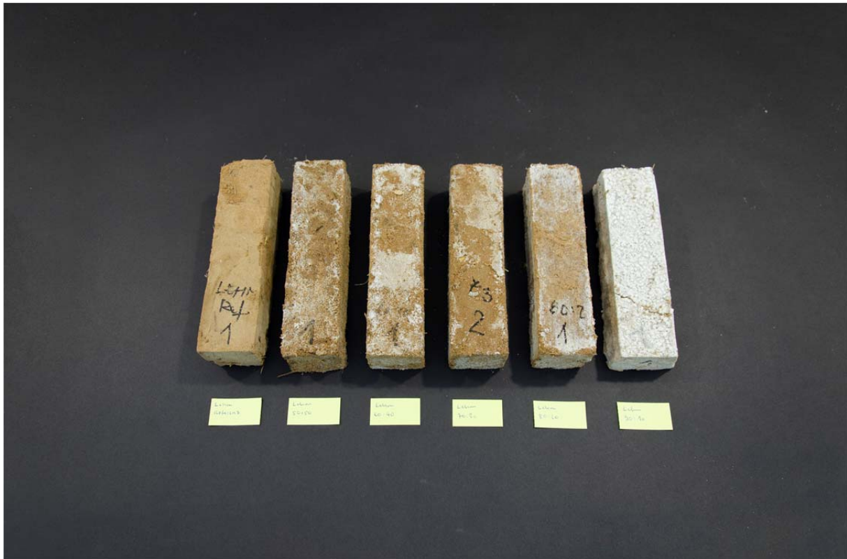
Figure 20. The salt and clay test specimens with different mixing ratios (from left to right): 0.0% salt + 100.0% clay, 10.0% salt + 90.0 % clay, 20.0 % salt + 80.0 % clay, 30.0% salt + 70.0% clay, 40.0% salt + 60.0% clay, 50.0 % Salt+50.0% clay.
