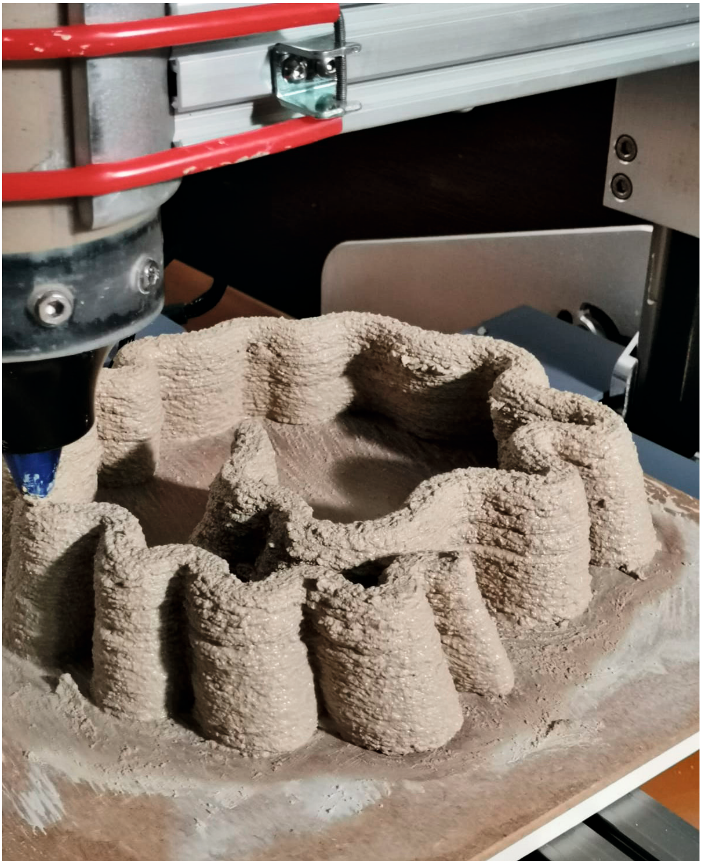
Figure 4. 3D printing with salt-clay paste.
