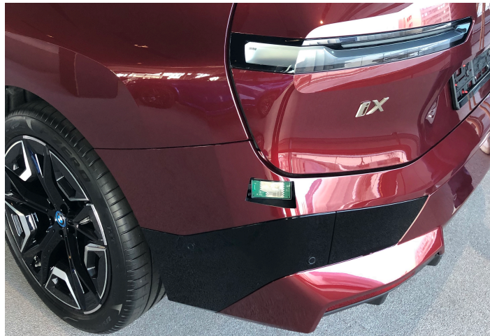
Figure 1.2: Cut away of SRR sensor integrated behind the painted bumper in the back.
