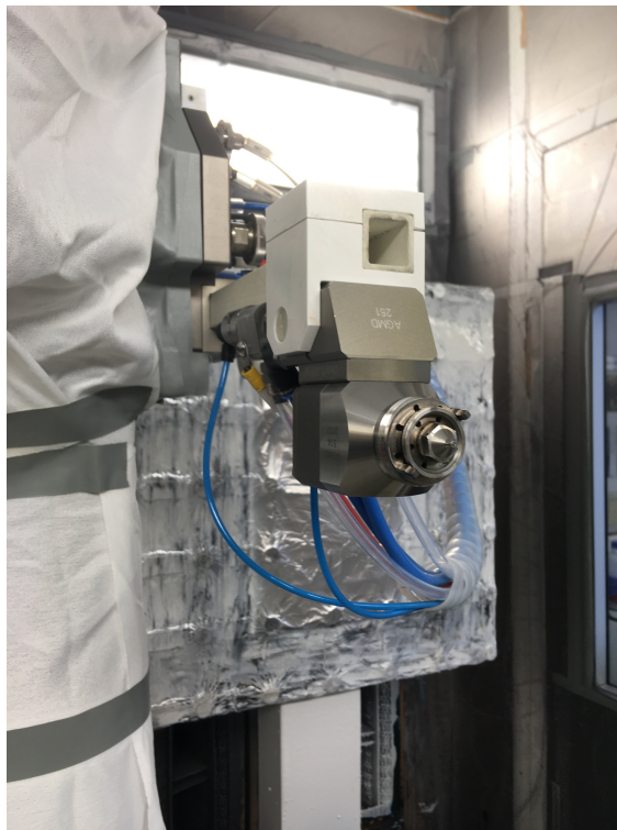
Figure 4.1: Pneumatic application system mounted on a robot. The air cap is removed, revealing the fluid nozzle in the middle.
