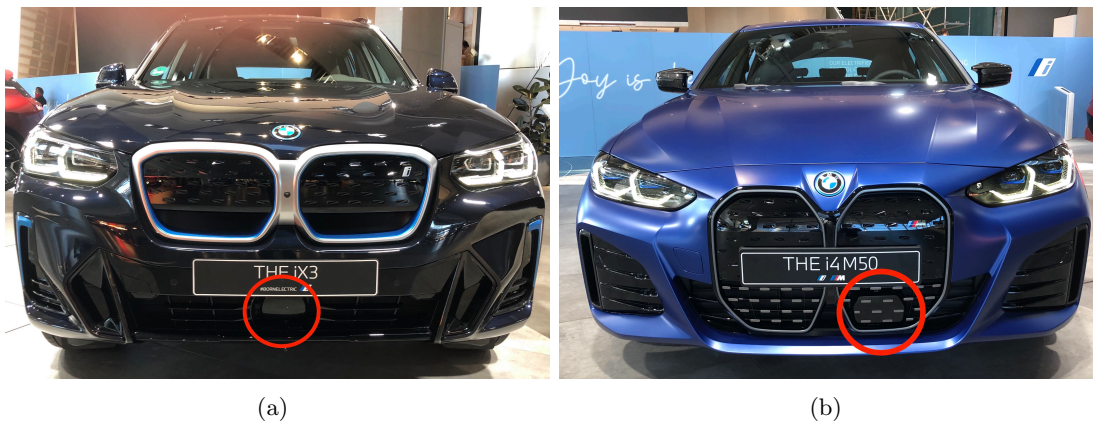
Figure 1.3: a) Radome of MRR for BMW iX3 located in the lower air intake b) BMW i4 radome with structure to match the design of the grill.
