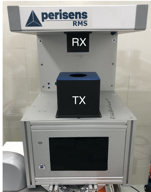
Figure 3.5: RMS measurement setup. The sample is placed on the hole on top of the TX antenna. In order to avoid measurement artefacts, the complete hole has to be covered by the sample.
