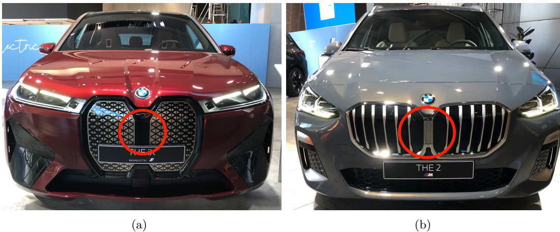
Figure 1.4: a) Multilayered Radome of BMW iX. b) Multilayered BMW 2 series integrated into the kidney grill. The middle part of the radome consists of a thin layer of indium in order to match the overall design.
