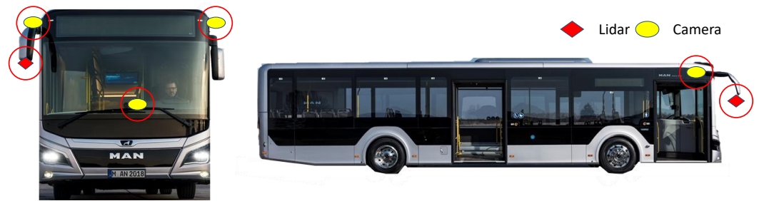
Figure 6. Test vehicle: a MAN Lion’s City 12 bus with positions for LiDAR and camera sensors.
