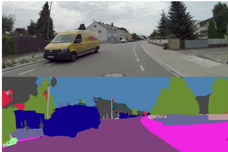
Figure 2. Top: original front camera image; bottom: semantic segmentation output of the given image using the ERFNet segmentation network [22].
