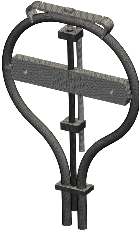
Figure 6.4: The mesh of the structural domain
