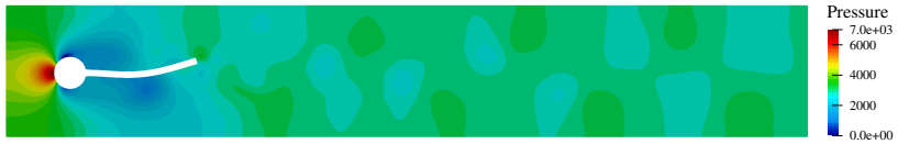
Figure 3.18: FSI3 benchmark: pressure contours at t = 19.743 s.
