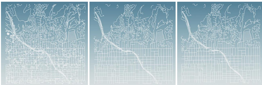
Figure 43: Left: Original OSM lines representing the streets. Middle: The street lines after the first filter. Right: The street lines after the second filter.
