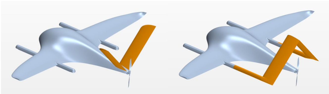
Figure 7: Left: V-tail (M2); right: inverted V-tail (M3)
