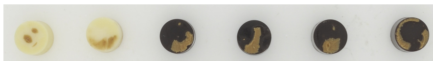
Figure 4.12: Picture of two cocoa butter, two chocolate and two 1:1-mixture cylinders (from left to right) with adherent nougat at the bottom (Sonnleitner 2016)
