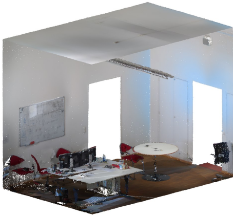
(a) Input point cloud of office (two walls are removed for better visualisation)
