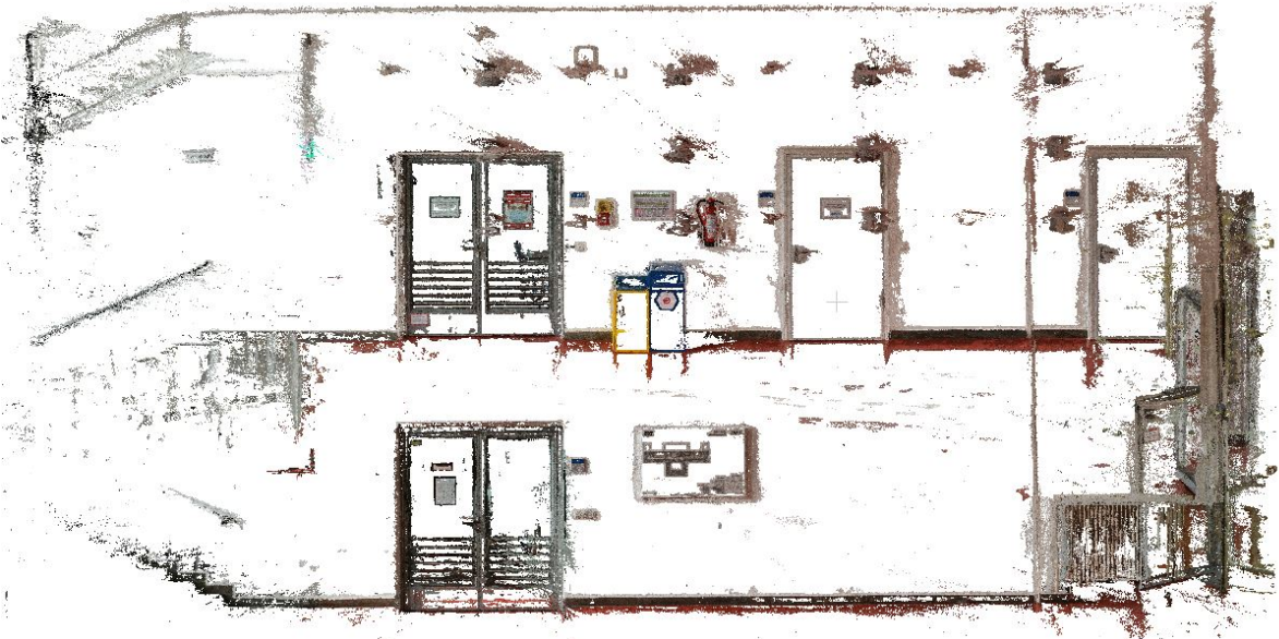
(b) Photogrammetric point cloud of indoor space
