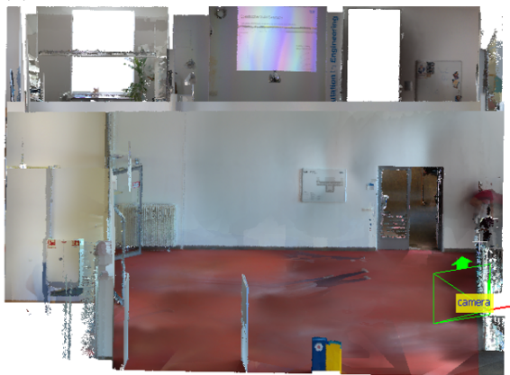
(c) Transform point cloud to camera frame (camera at origin)
