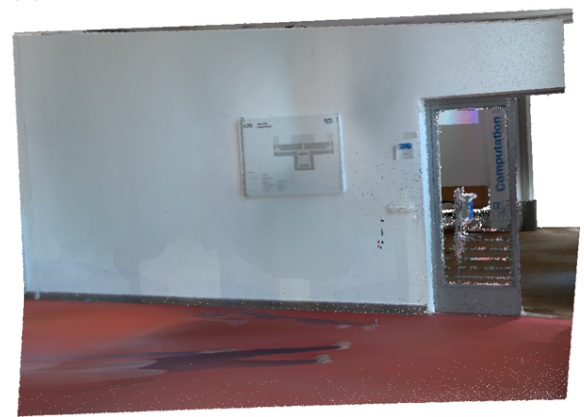
(d) Visible points from laser-scanned point cloud at camera pose
