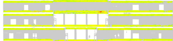
(e) Filtered point cloud with n_1 = 10
