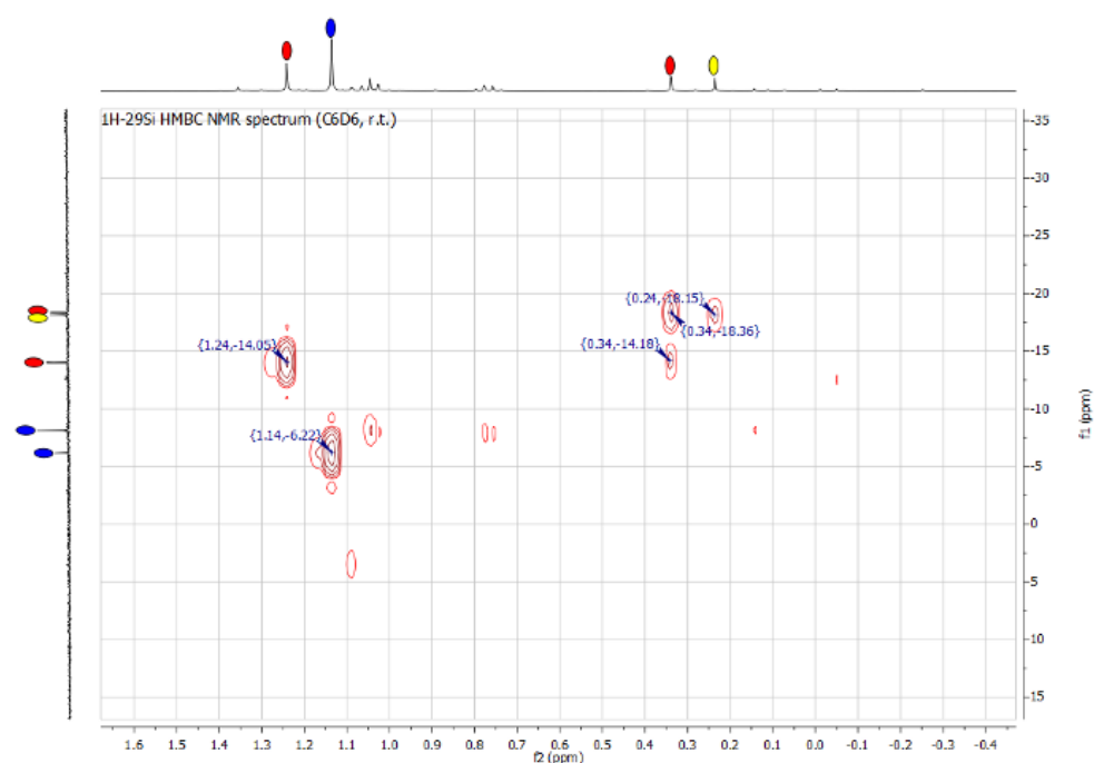
Figure S32. 1 H- 29 Si-HMBC (500 MHz/100 MHz, C 6 D 6 ) of photoreaction of E14 , with the insertion (blue), eliminated acetylene (yellow), and rearrangement (red) product mixture.
