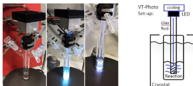
Figure S26. Irradiation set-up for all photoreactions. Additional covers were arranged to protect the staff from harmful UV-light. Schematic layout of the setup (right) and actual images of the setup (left).
