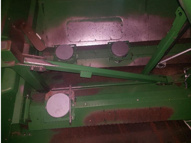
Figure 6: Load cells in the grain tank (JOHN DEERE 2019)
