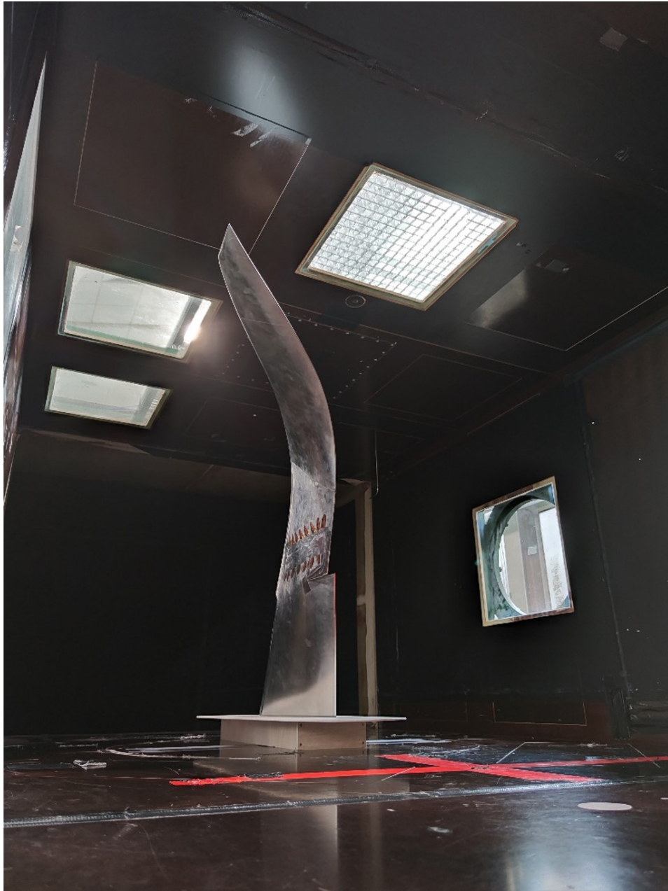
Figure 5.10.: Outer Winglet Model installed in the wind tunnel [219].
