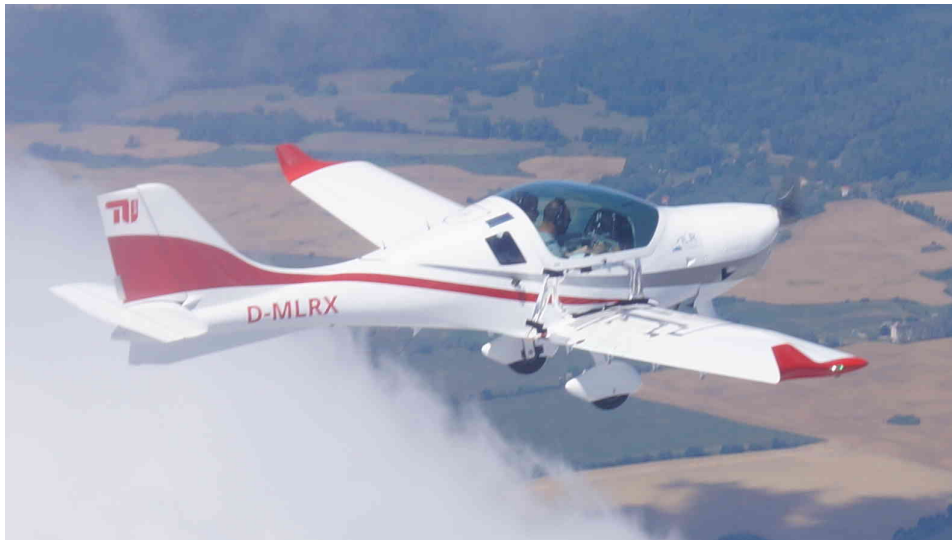
Figure 5.23.: Test aircraft with instrumentation in flight. Test aircraft is instrumented with fiber-optic pressure sensors on its right-wing [217].
