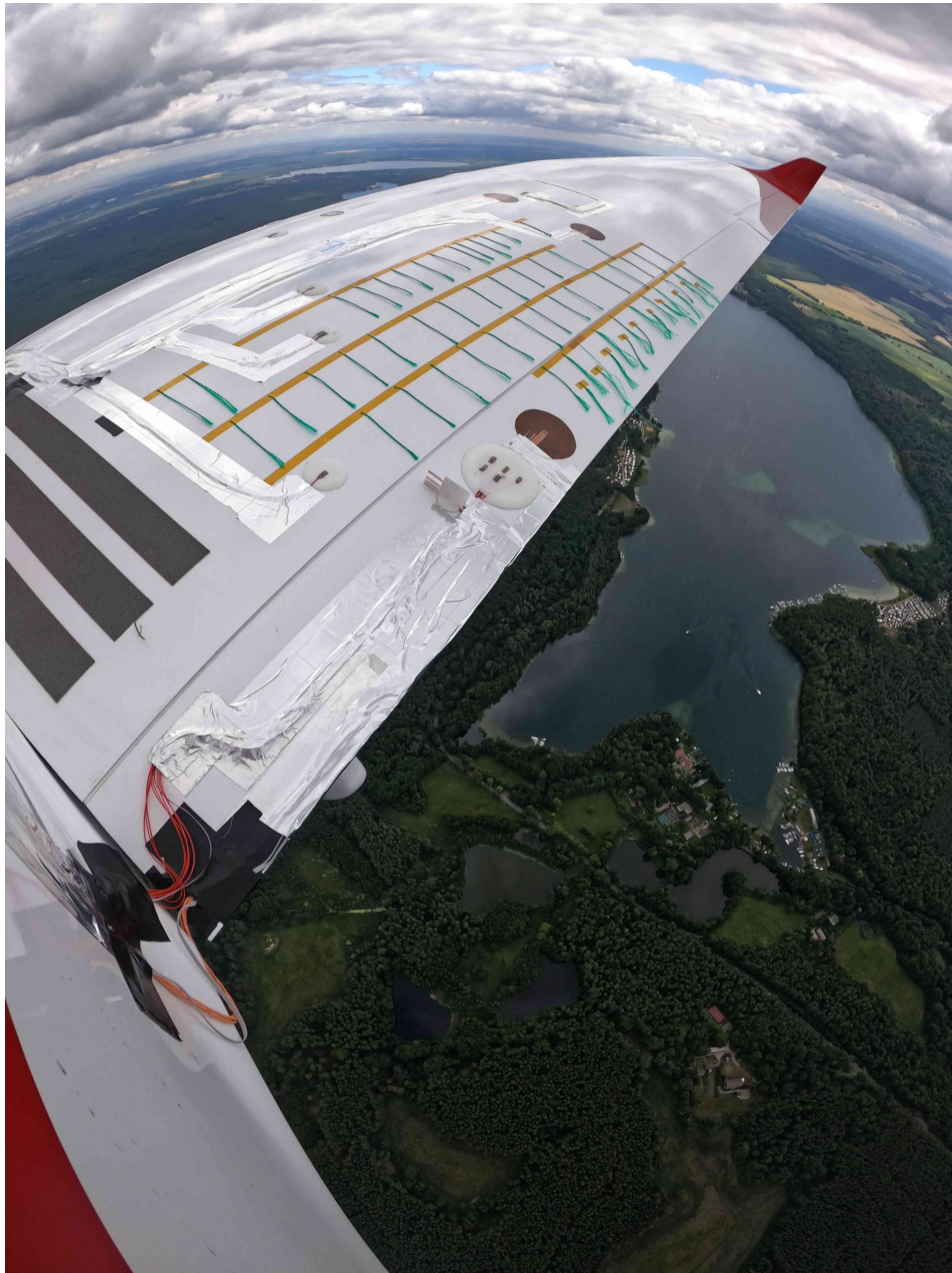
Figure 5.25.: Cockpit view on instrumentation. In this picture, the aircraft is airborne and climbing above the Werbellinsee, north of Berlin, Germany. The figure shows the instrumentation. The fiber-optic sensors are installed across the airfoil with a concentration on the flap. The cables are taped to the airfoil. In order to route the cables along the movable flap, the cables have been mounted in a loop near the mainframe. This routing of the fibers allows them to expand. The extra green chords are installed to illustrate the airflow direction and are monitored with a video camera during flight. Other electrical sensors have been installed next to the fiber-optic equipment for other research and benchmark purposes [217].
