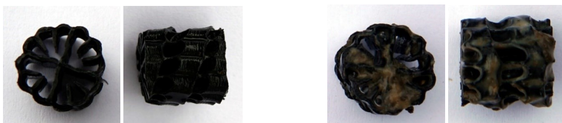
Figure 9-5: Sampling of the biofilm carrier from the bottom of the packing bed (left) and from the top (right) after 447 days.
