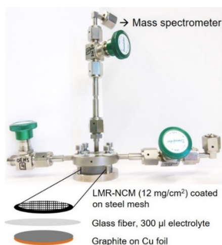
Figure 15: Adapted OEMS setup of Tsiouvaras et al. 104 that shows the OEMS cell used for measurements done in this thesis. The middle part hosts the cell stack that consists of a conventional anode, the separator, and the cathode. The cathode in this setup is not coated as usual on aluminium foil but on a stainless steel mesh to allow unhindered gas transport from the bottom of the cell to the capillary. More details about the used setup in this thesis can be found in the experimental section in the article by Schreiner et al. 63 The headspace of the cell is around 10 ml. The tubes right and left can be closed by the green valves, which allows the flushing of the cell with either a calibration gas or argon. The capillary is indicated and connects the cell with the mass spectrometer system.
