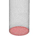
Reactor mesh and CFD simulation of air staging
