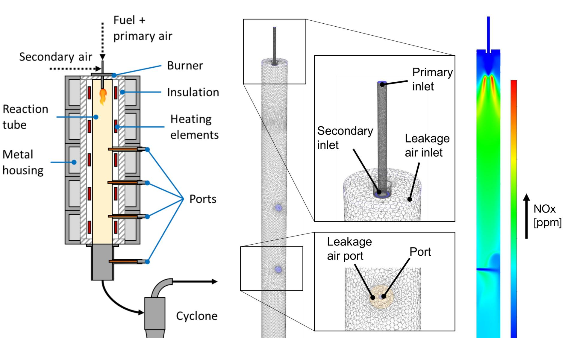
Up-scaling simulations to medium-sized biomass boilers
