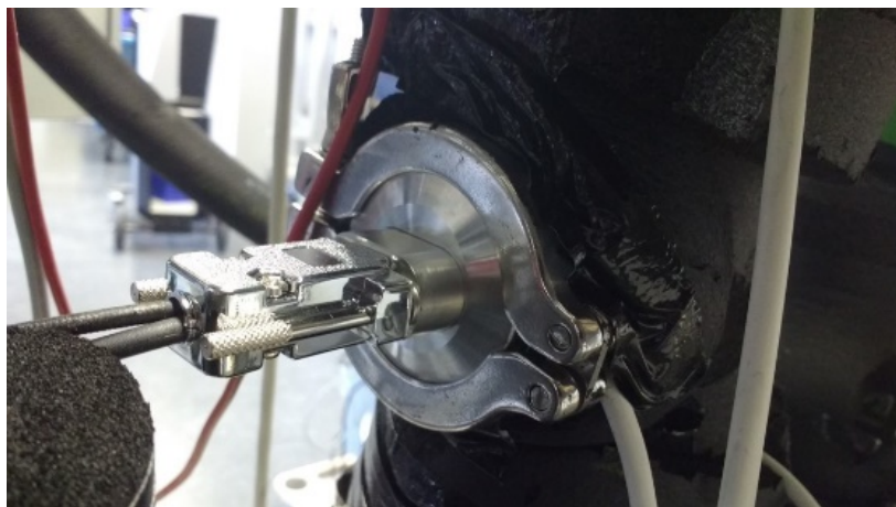
Fig. 8.2 Vacuum feedthrough of the two endoscope cameras into the test unit
