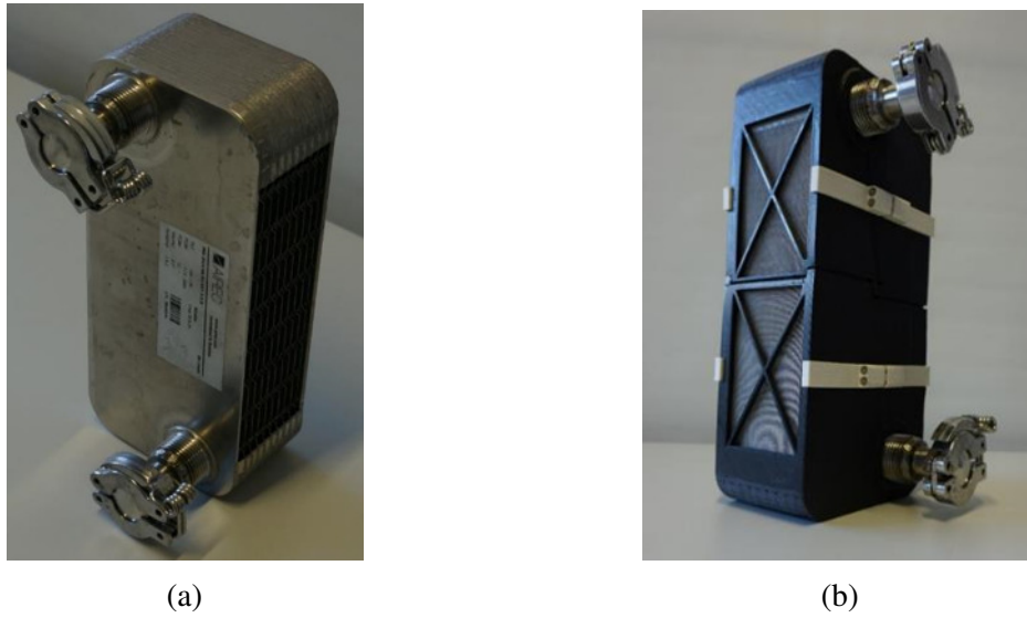
Fig. 3.1 The GLX30 adapted as an adsorber heat exchanger (The open sides for vapour flow into/out of the adsorbent domain are covered by a stainless-steel sieve to prevent the loose pellets from falling). (a) Before being filled in with the adsorbent, (b) adapted and filled in with Siogel grains.
