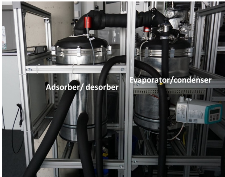
Fig. 3.3 Realized test setup for investigating the APHE at the LSP of OTH-Regensburg, Germany.
