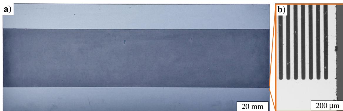
Figure 4.6: a) Photograph of the fabricated grating #1 with an active area of 170 \text{ mm} \times 38 \text{ mm} . b) A magnified image of the lower right grating edge acquired with a light microscope. The grating lines are parallel to the short edge of the grating.
