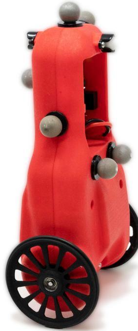
Figure 1.1: TWIP with markers for an optical tracking system
