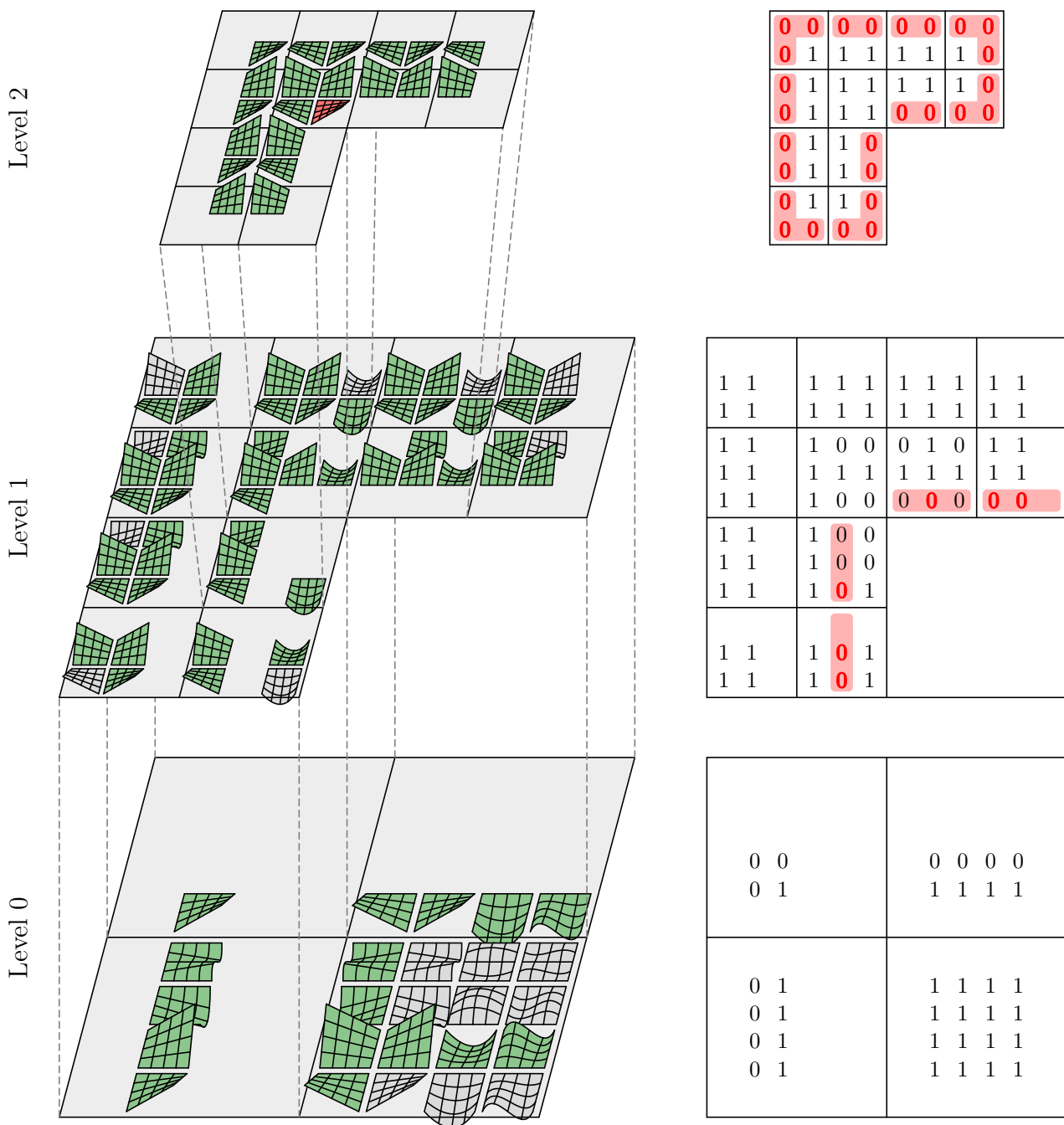
Figure 4.7: Deactivate internal boundaries (step 3). From Kopp, Rank, et al. (2022), used under Creative Commons CC BY 4.0 license.
