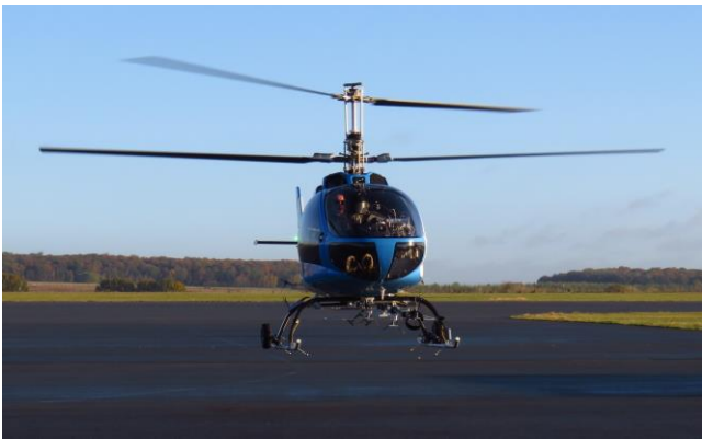
Figure 1: Front view of the test aircraft with air data boom, antennas and ground contact switches visible on the landing skid and the avionics system rack on the copilots' seat
