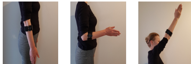
Figure 7. Limb poses included in the experimental protocol. Limb poses and corresponding angles from left to right: pose 1°—0°, shoulder and elbow flexion, pose 2°—90°, elbow flexion, pose 3°—135°, shoulder flexion.
