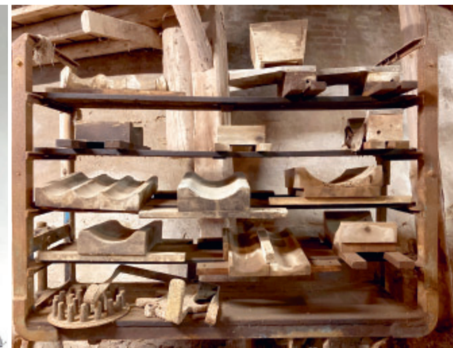
Fig. 4: Moulds and tools for terracotta production, Lilleskov Teglværk, Denmark (Asha Sumra and Arijit Chatterjee, June 2022)
