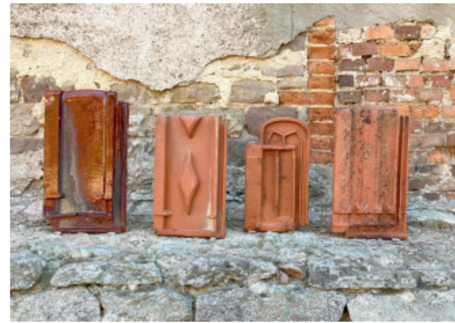
Fig. 3: Mechanical tiles still in production at Tuilerie de Niderviller, France. Including flat tile, Gilardoni tile and Marseille tile (Asha Sumra and Arijit Chatterjee, June 2022)
