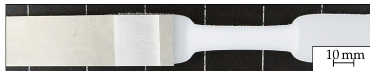
Figure 5. Typical FPJ tensile shear test specimen made of PE-HD and EN AW-6082-T6 (I-PSd) after a successful lap shear test with distinct strain hardened area.
