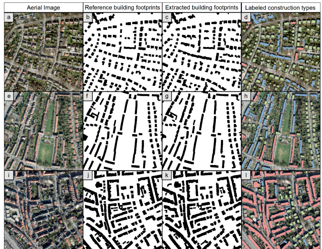
Figure 5. Results of the building extraction using U-net Inceptionresnetv2 for various building morphologies in the city of Münster. Aerial images as input data are depicted in (a,e,i), reference building footprints from the official LoD-1 building model are shown in (b,f,j), results of building footprint extraction are presented in (c,g,k), and the result of labeled construction types is displayed in (d,h,l).
