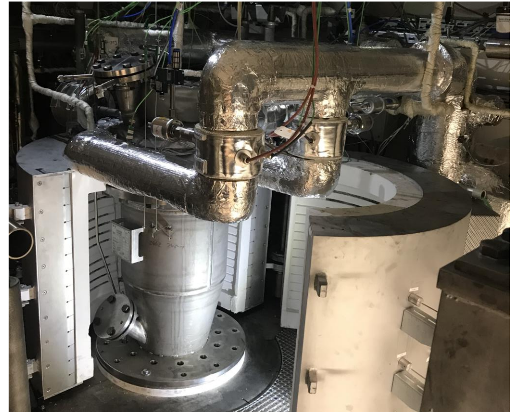
Freeboard and off-gas-system of the pilot-scale reactor FluBESToR
