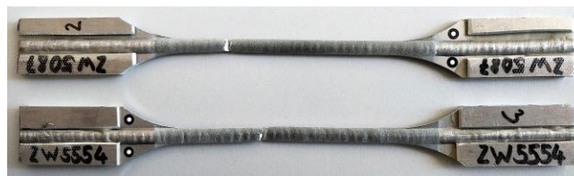
Figure 2: Tensile samples consisting almost exclusively of weld metals AA-5087 and AA-5554, shown after tensile testing.
