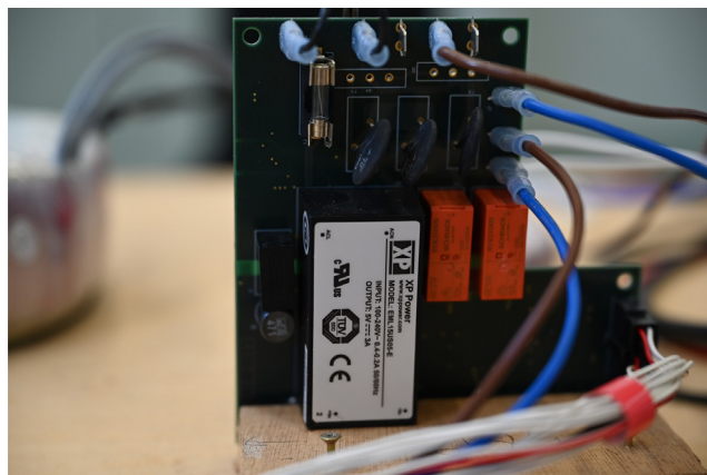
Fig. 29. System Input System Output board with the 14 pin WR MPC3 connector to DISP. The two left flat plugs on the top side connect SISO to the primary side of the high voltage transformer and the flat plugs around the top right corner to the primary side of the high voltage power transformer. The other two flat plugs connect the SISO to the 230V inlet of the PLUSPULS.
