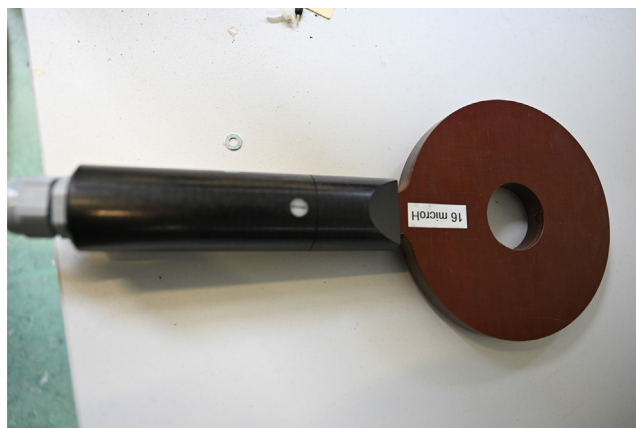
Fig. 36. Stimulation coil with inductance of 16\mu\text{H} used for the stimulation.
