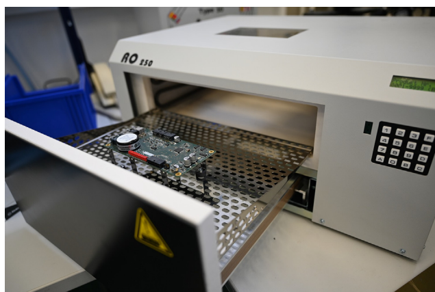
Fig. 20. PCB (already finished) placed in the reflow oven ready to start the temperature curve to solder the SMD components on the PCB.
