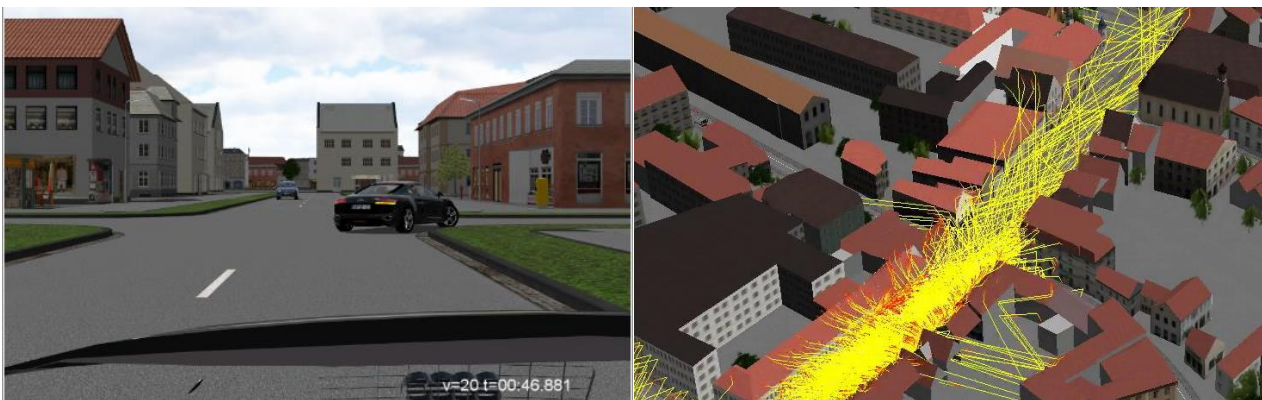
Fig. 1: 3D-visualization of the submicroscopic traffic and vehicle simulator Virtual Test Drive (VTD) and a real-time electromagnetic wave propagation simulation of Car-to-Car-Communication within VTD (SCHILLER et al. 2014).
