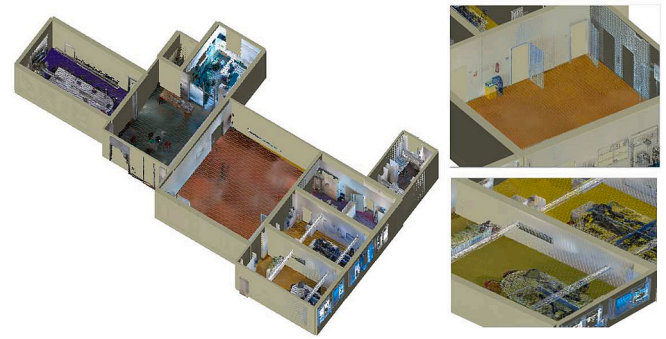
Fig. 17. The process of fitting the highly parameterized digital model to the point cloud dataset (the ceiling points were removed to improve the visual representation).
