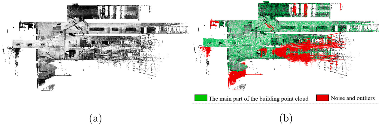
Fig. 5. Filtering of the noise and outliers using the CCS method: (a) raw point cloud data, (b) the result of filtering noise and outliers.
