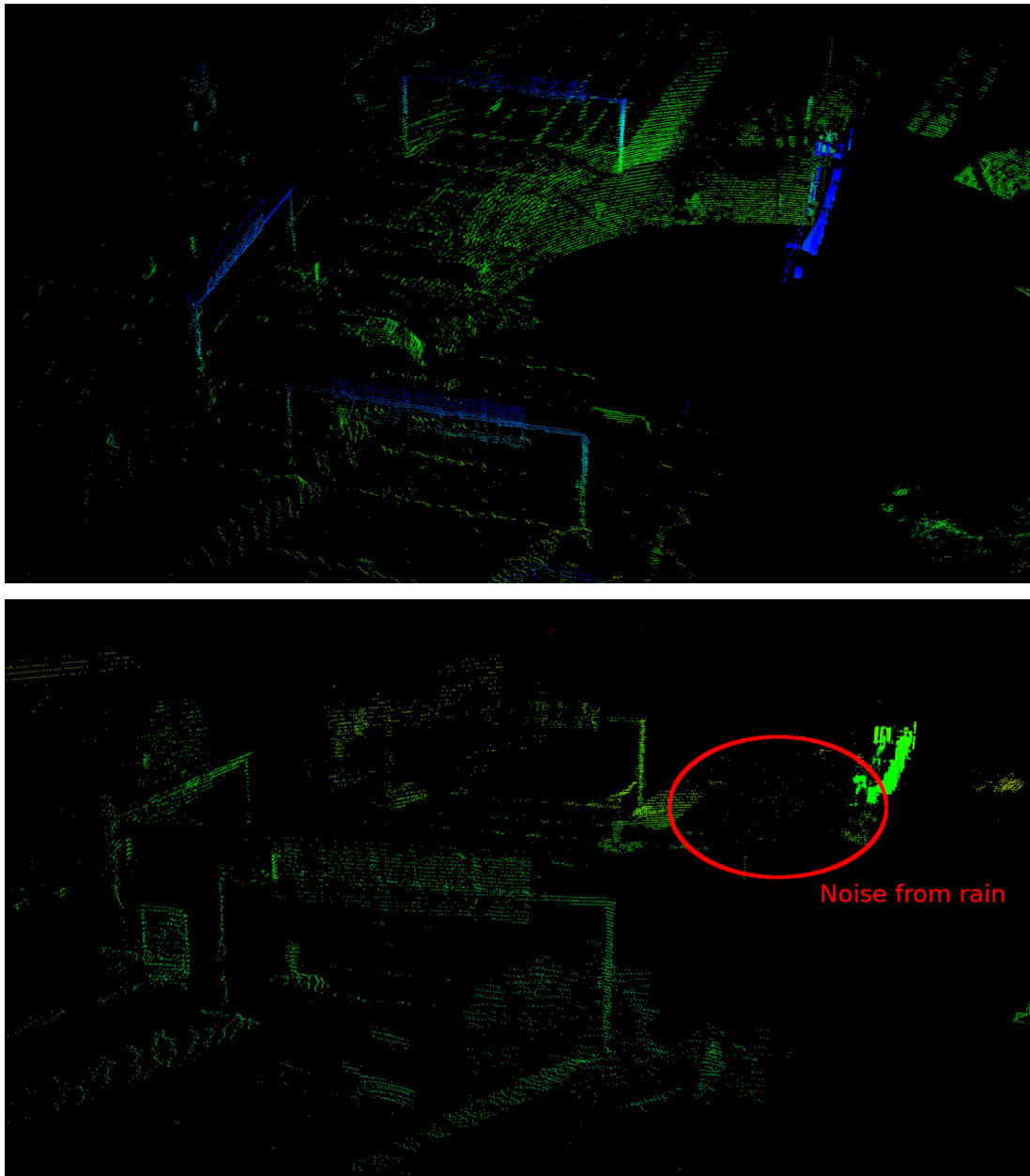
Figure 1.6: Point cloud from dry and rainy weather. Not only is the point cloud from rainy weather noisy, but it also contains \sim 60\% fewer points than the point cloud from dry weather.
