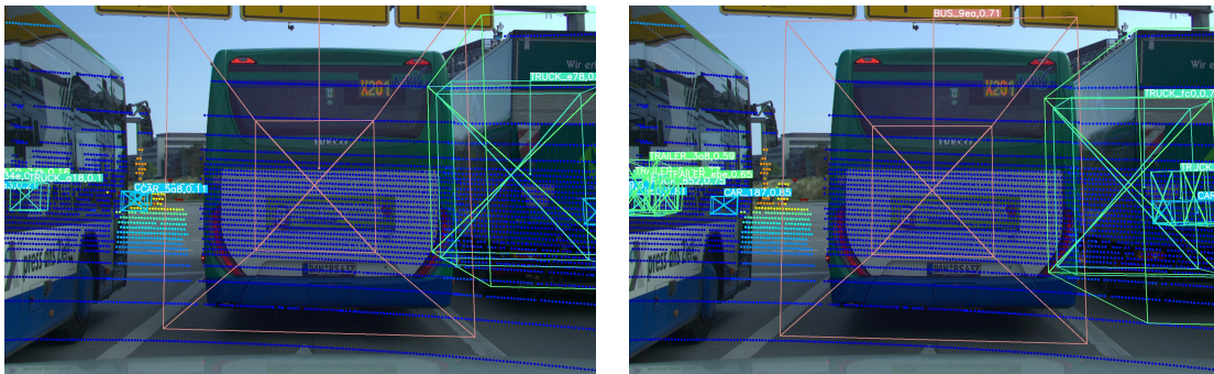
Figure 6.1: Occlusion set 1, vehicle POV: vehicle-only vs. cooperative. The detections beyond the three large vehicles shown in the vehicle-only case are all misplaced and inaccurate as shown in Figure 6.2. This is likely only possible due to the overfitting causing the model to guess/estimate object class and locations even when there are no points. Meanwhile, the low score threshold of 0.1 allows the objects to become false positives.
