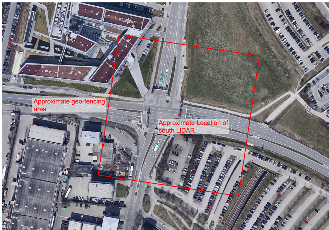
Figure 3.1: S110 intersection with the approximate point cloud geo-fencing area and the approximate location of the south LiDAR, which serves as the origin of the infrastructure coordinate system.
