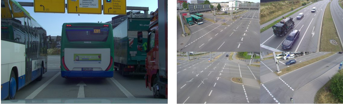
Figure 1.2: Occlusion problem from vehicle and infrastructure POV images. While the vehicle could not see anything beyond the three large vehicles in front of it, infrastructure based sensors could clearly see everything.
