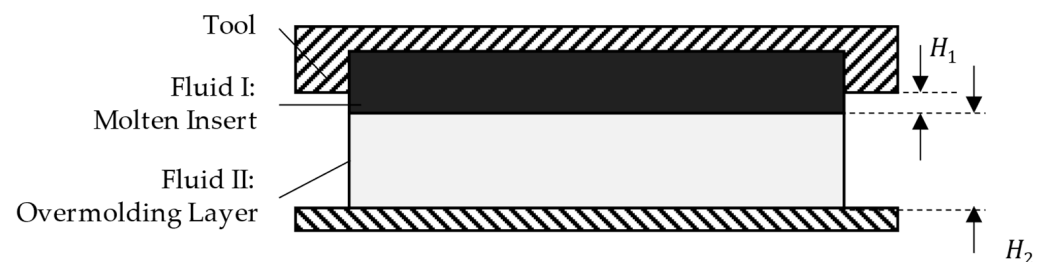
Figure 9. Schematic representation of an overmolding setup with an overmolding layer and an insert, where part of the insert height is covered by a tool.
