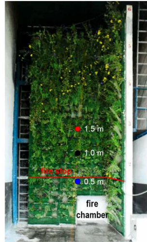
Figure 6. Temperature–time diagram (left) in the rear-ventilated void cavity in different heights [0.5 m above the fire chamber (under fire stop), 1.0 m and 1.5 m above the fire chamber (above fire stop)]; photo of the test stand with arrangement of the measuring points in the rear-ventilated void cavity; based on [101].
