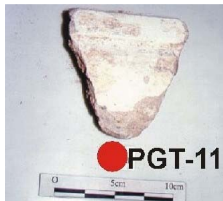
Figure 75. Sampling of the surface layer of white moulded stucco.
