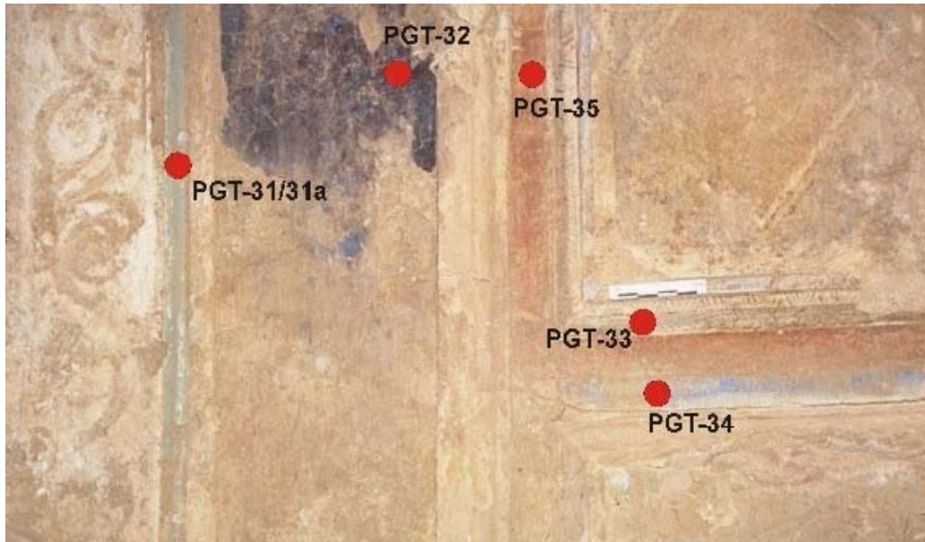
Figure 78. Sampling of the moulded stucco along the south corridor wall.
