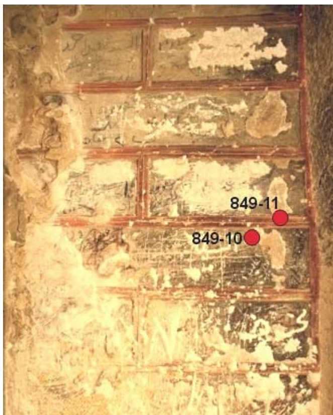
Figure 39. Sampling from the stucco covering the back wall of the biclinium.
