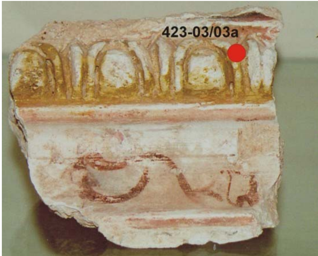
Figure 85. Sampling of a stucco surface covered with gold leaf from the Temple of Winged Lions.
