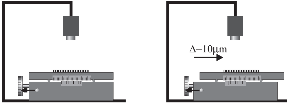
Figure 4.31: To test the accuracy, the IC was mounted on a precise xy\phi -stage, which can be shifted with an accuracy of 1\ \mu\text{m} and can be rotated with an accuracy of 0.7' ( 0.011667^\circ ).
