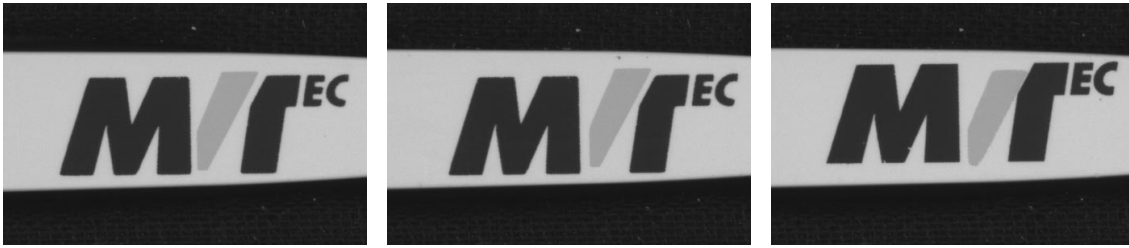
Figure 2.6: The logo “MVTEC” is an example of a compound object that consists of the two object parts “M Tec” and “V”.
