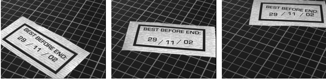
Figure 3.6: Deviations from the nadir view cause projective distortions in the object plane.
