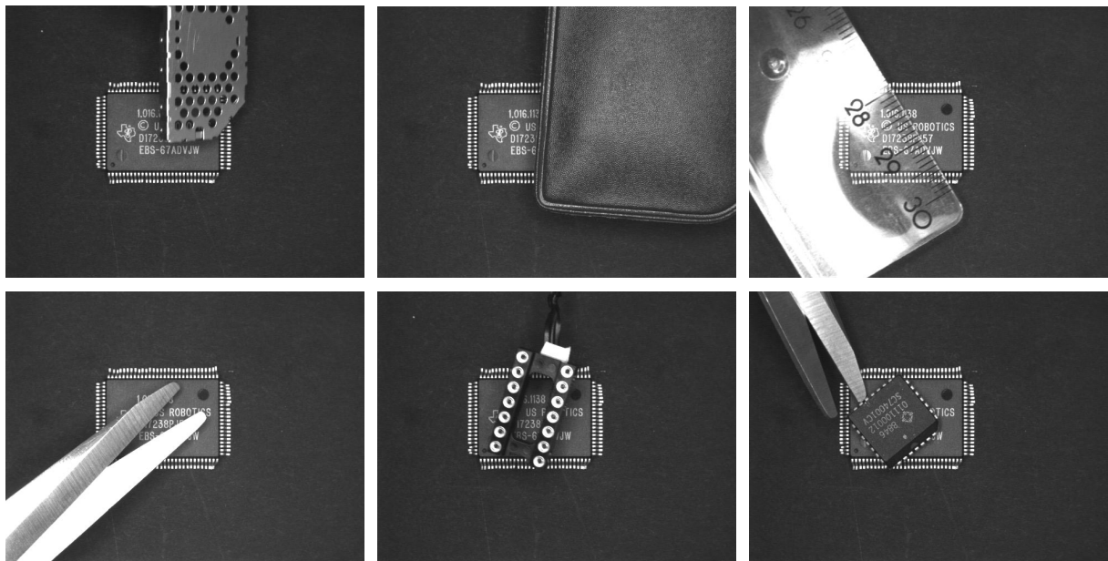
Figure 4.23: Six of the 500 images that were used to test the robustness against occlusions
