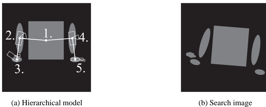
Figure 5.25: A compound object consisting of five object parts. In (a) the hierarchical model is visualized. Additionally, the position in the search order of each part is displayed. In the search image (b) a clutter object is present.
