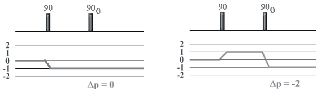
Figure 2-2: A pulse sequence of 2D-COSY experiment with P (left) and N (right) type coherence transfer pathways.
