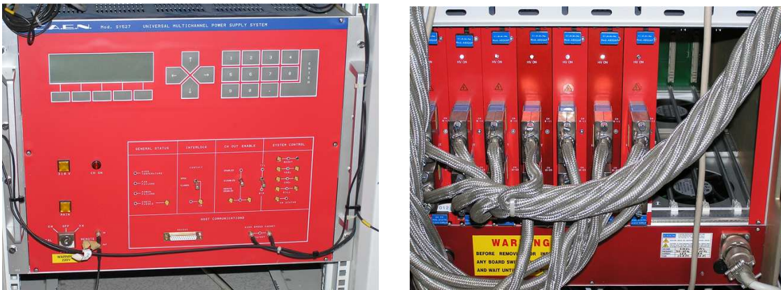
Fig. 4.2: CAEN SY527 Mainframe. Front View (left) and rear view (right), where seven A932AP boards are visible.
