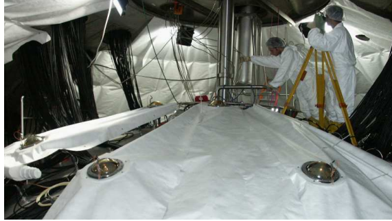
Fig. 3.13: Topographic survey: one of the stations on top of the SSS.
