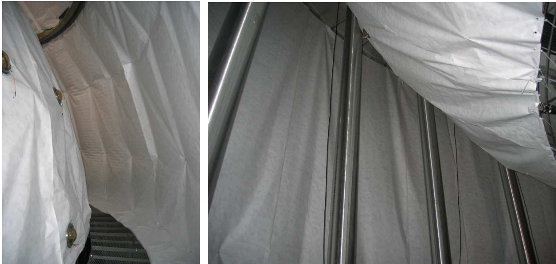
Fig. 3.9: Pictures of the water tank: upper (left) and lower (right) outer detector segments are covered with Tyvek sheets. The walking grid will also be covered before WT closure.
