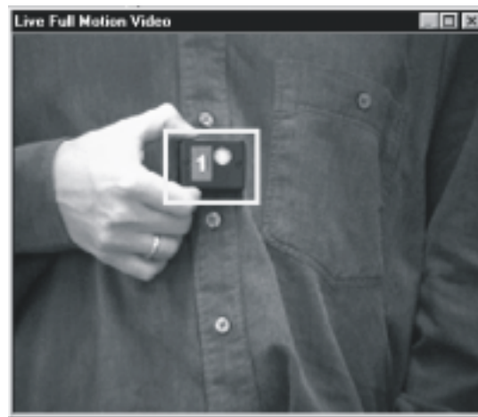
Figure 5.9 Video picture of a tag with the overlaid position information.
