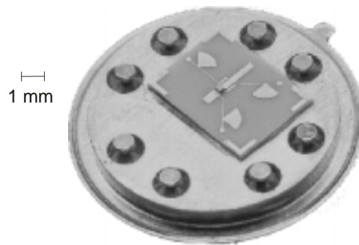
Figure 4.3 Free running AIA mounted on a gold header.
